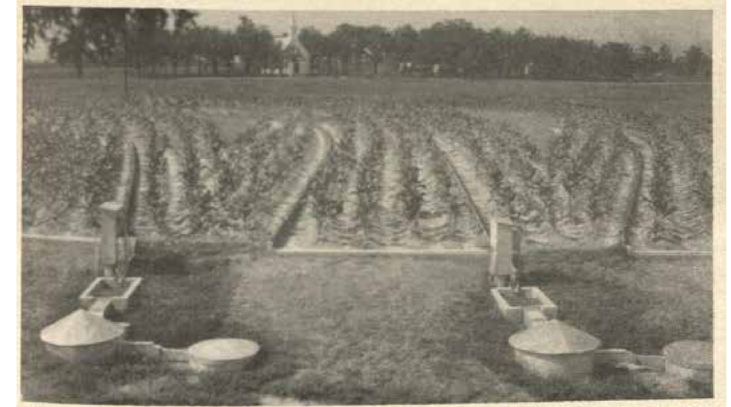
Figure 1. Runoff plots and catchment equipment from which soil and water loss measurements were made.
